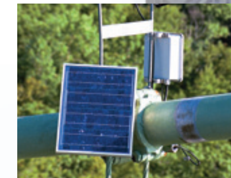
State-of-the-art solar-powered wireless sensor technology eliminates the need for data communications cabling, and further reduces installation.
