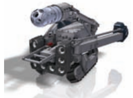
Robotic device used to inspect the water main
